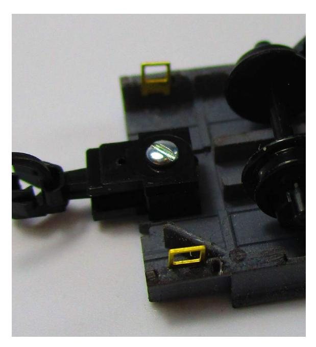
3. Now move on to the bulkheads. Bend the end walkways down so the pins project backwards. Glue these parts in place. (The bulkheads are identical.) Be careful while doing this bending and take your time, as the etched parts are delicate. I used a toothpick to apply some glue to the etched parts, then stuck them in place. You can see I already pinned the bottom of the ladder assemblies to the bulkhead with grab irons. Don't install these until later.
