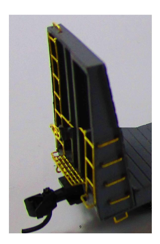
8. Glue in the handbrake chain, through the notch in the end sill, and up behind the handbrake housing.
