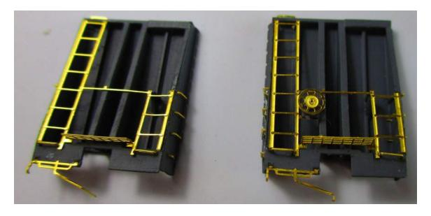
Glue the bulkheads to the body, ensuring they are straight with a square. Before gluing, make sure that they are fully seated as well. Remember- the bulkhead with the brake wheel goes on the end of the car with the brake lever assembly and small notch in the end.
