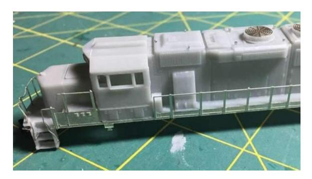
7. Insert the couplers into the shell, and screw them in place with the screws included with the MT couplers. Glue the ditch lights to the pilots, and the plow to the front pilot. This photo shows the number boards installed, but we recommend you leave these off, paint them seprately, and install after painting. At this point, you can install the step lights if you wish to use them. They are tiny and almost invisible but they're included!
