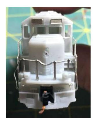
8. Install these parts after painting- windshield wipers, cab door handles, number boards, and cab side windows.
