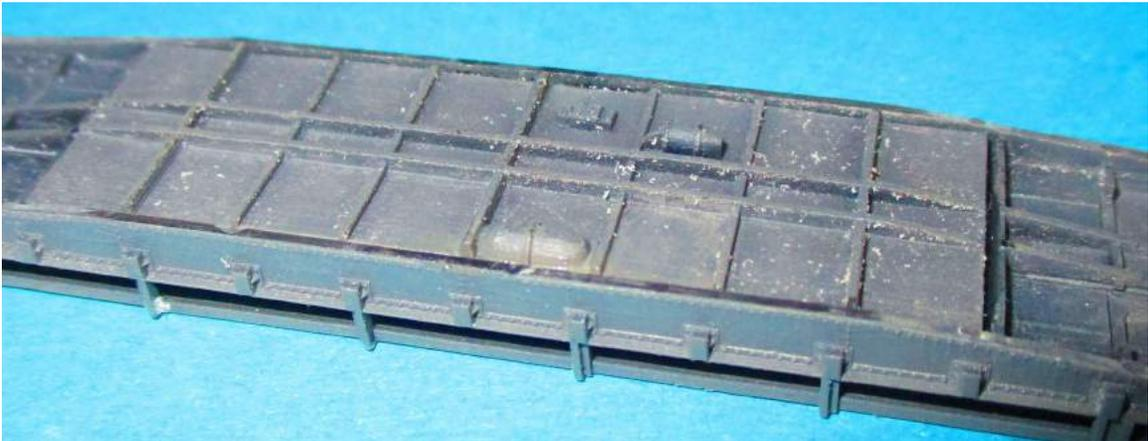
6. Remove the brake rod assembly from the fret and glue it to the underframe.
