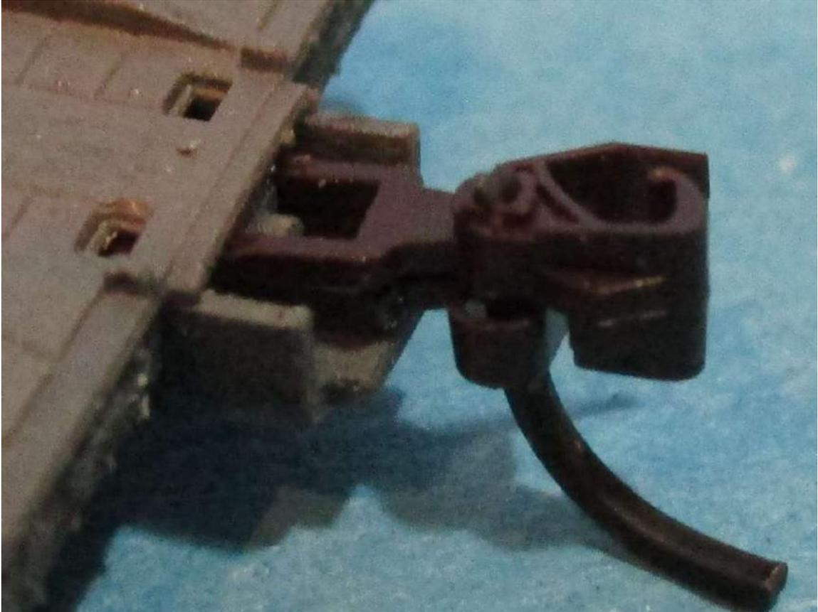
4. Insert the coupler springs into the boxes, then push the couplers the rest of the way in.
